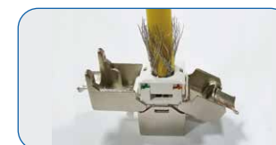
3.Placing the cable into the IDC cover.
